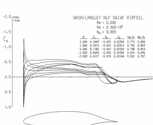
Fig 6: Pressure Distribution over a NLF-0414F wing for various AOA varying from 2 degrees to - 2 degrees @ Re 300000 (XFOIL 6.94)
