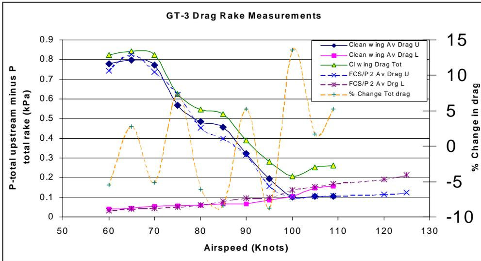
Fig 10. Profile drag contributions from upper and lower surfaces on GT-3 wing
