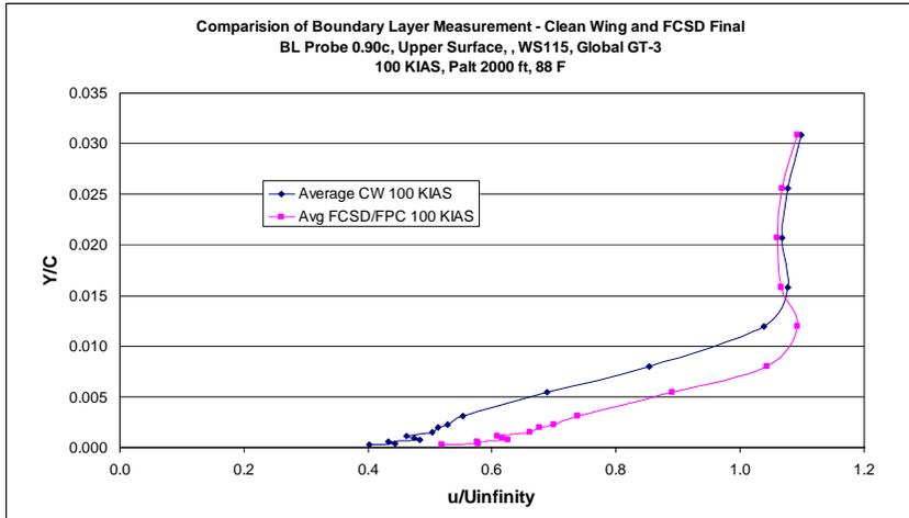
**Fig 11b: Suction surface boundary layer velocity profiles at 100 KIAS on a GT-3 Aircraft wing at 0.90c**
