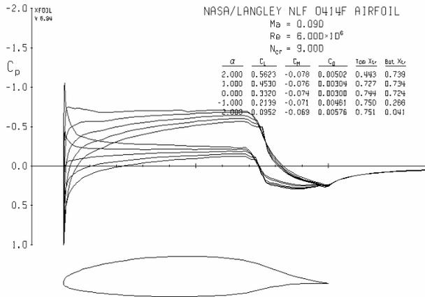
**Fig 9: Pressure Distribution over a NLF-0414F wing for various AOA varying from 2 degrees to -2 degrees @ Re 6-million (XFOIL 6.94)**
