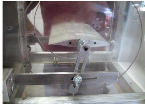
**Figure 2: Sinhatech Slow-speed Wind-Tunnel**      **Figure 3: Close up of tunnel section showing the NLF-0414F airfoil**
