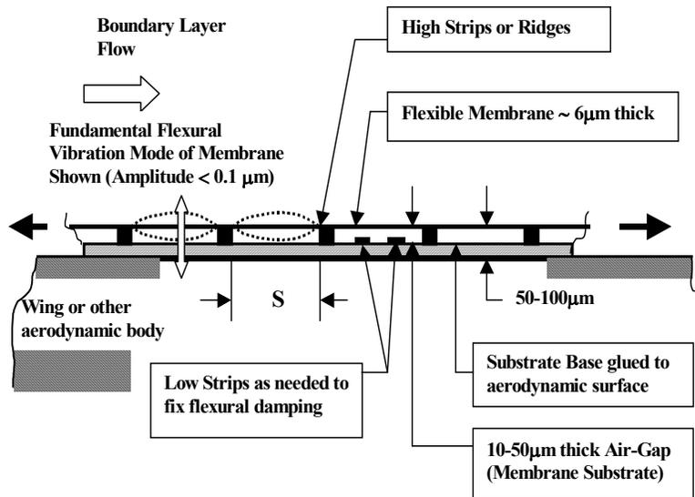
**Fig 1a. Schematic of the SINHA Flexible Composite Surface (FCSD)**
