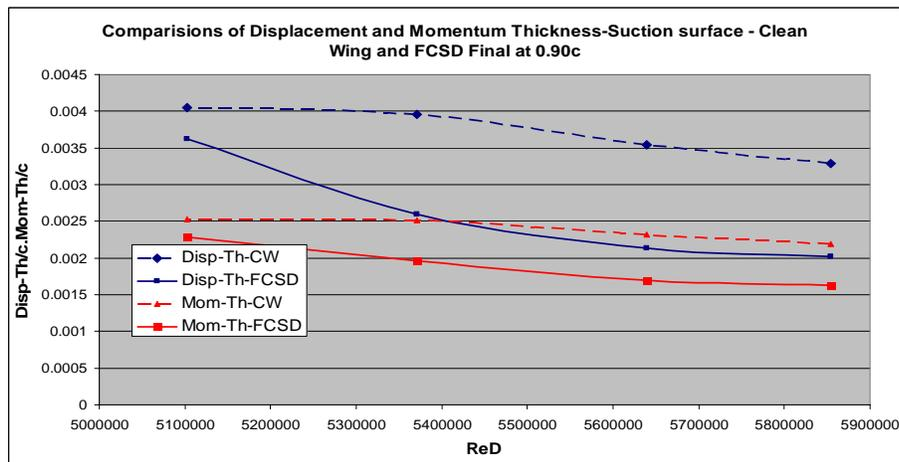
Fig 13: Comparison of Displacement thickness and momentum thickness at 0.90c on the suction surface of a GT-3 Wing
