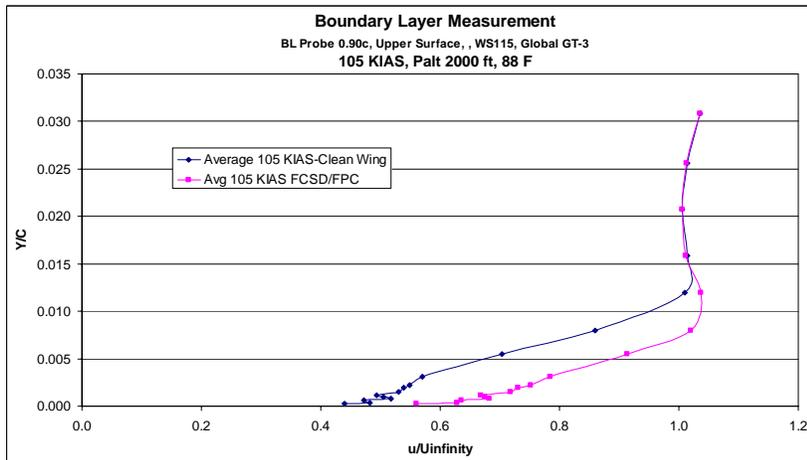
**Fig 11c: Suction surface boundary layer velocity profiles at 105 KIAS on a GT-3 Aircraft wing at 0.90c**
