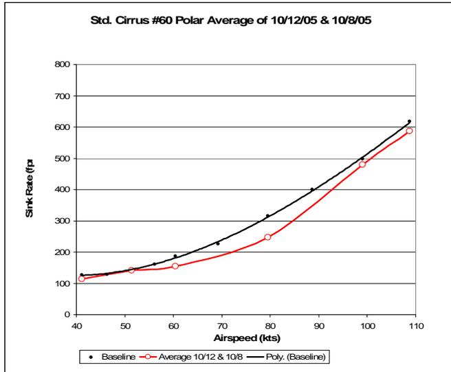
**Fig 14. In-Flight Sink-Rate (top) and L/D measurements (bottom) of a Standard Cirrus Sailplane with Wortmann “natural laminar flow” airfoils, with (red) and without (black) full-span upper-surface FCSD treatment**
