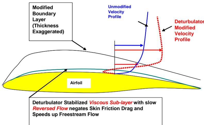
Fig 15. Sketch showing how FCSD reduces drag by maintaining thin stable separated regions.
