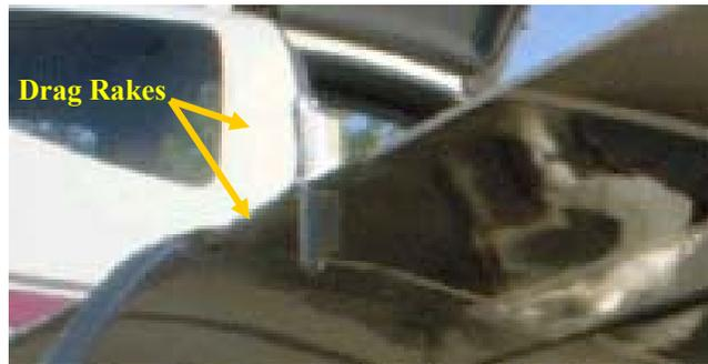
Figure 4: Drag rakes mounted on the trailing edge of the GT-3 wing
