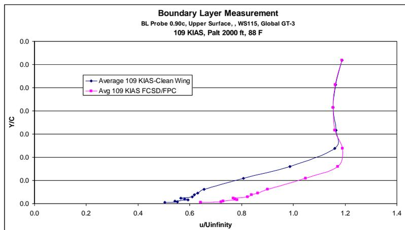
**Fig 11d: Suction surface boundary layer velocity profiles at 109 KIAS on a GT-3 Aircraft wing at 0.90c**
