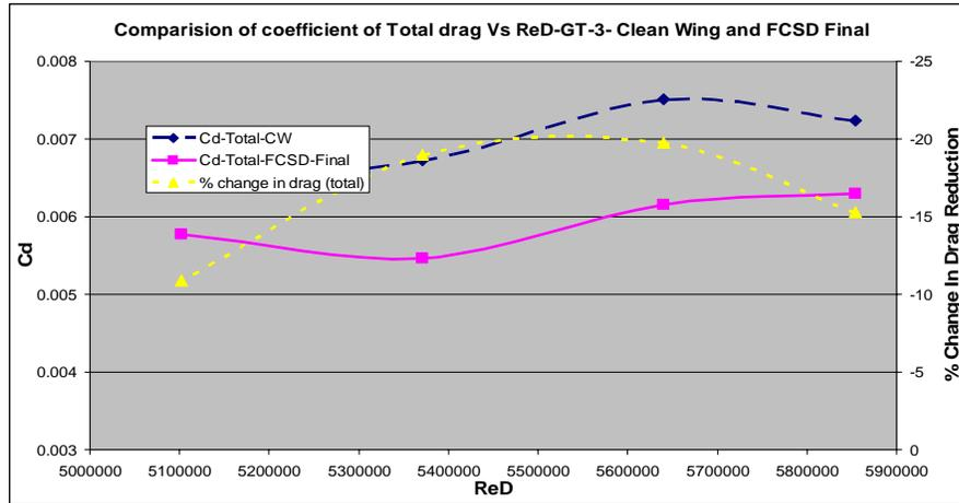
Fig 12: Comparison of total drag Vs Re – Clean wing and wing with FCSD
