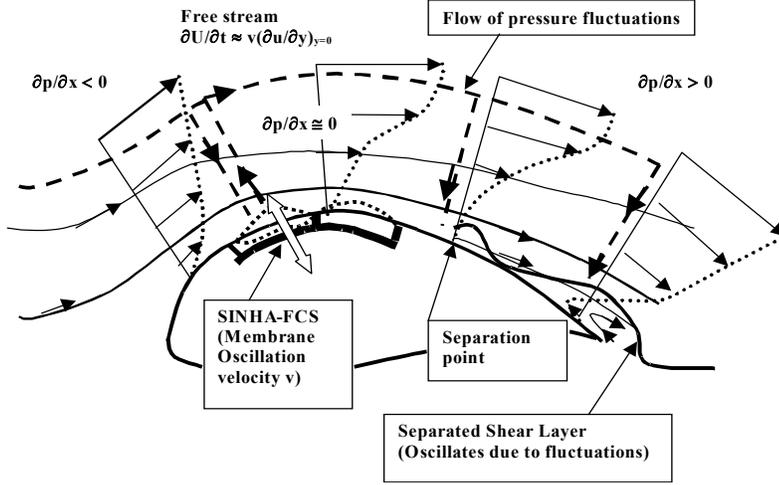
**Fig 1c. Schematic of the interaction of the SINHA-Flexible Composite Surface with a streamwise varying pressure gradient boundary layer on an airfoil. Thickness exaggerated for clarity.**
