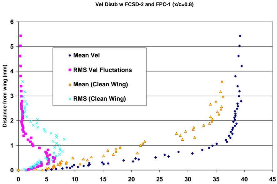
**Fig 8. Boundary Layer Velocity Profiles at  $x/c = 0.8$  on top surface of NLF-0414F wind tunnel model ( $Re = 0.3M$ ,  $\alpha = -1^\circ$ ,  $M = 0.09$ ) with and without FCSD-2**
