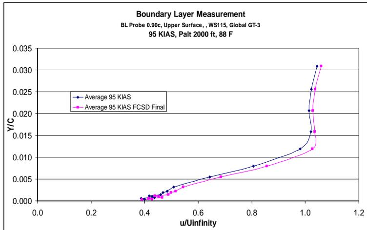
Fig 11a: Suction surface boundary layer velocity profiles at 95 KIAS on a GT-3 Aircraft wing at 0.90c
