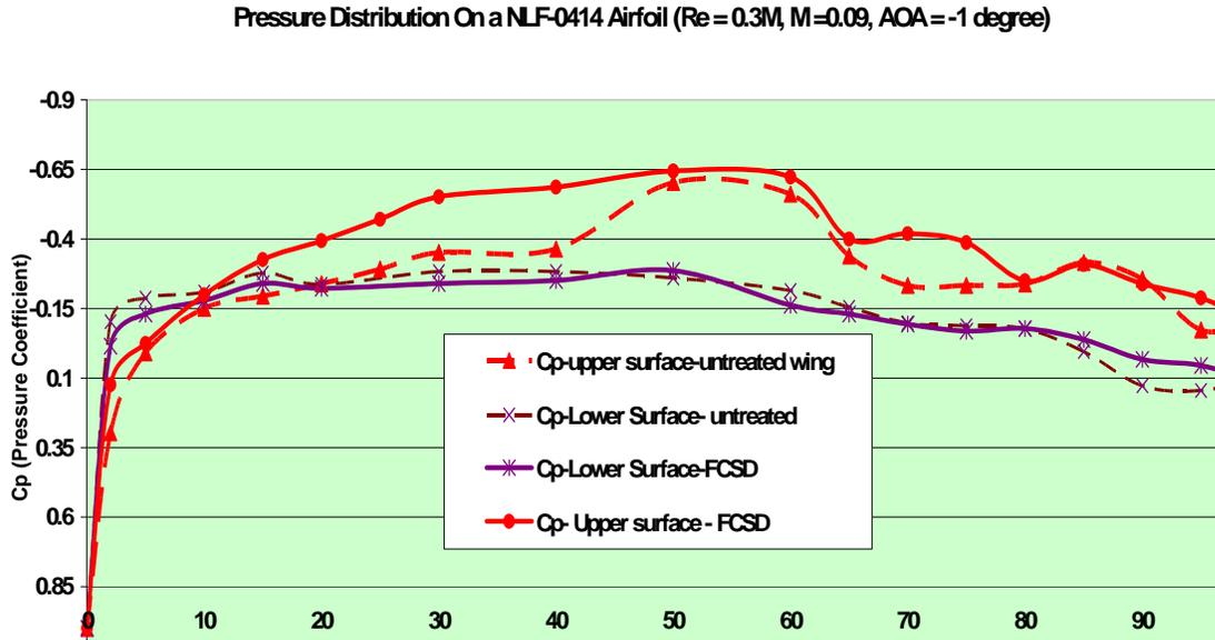
Fig 7: Pressure Distribution on NLF-0414F airfoil model tested in the SINHATECH wind-tunnel showing the effect of FCSD flow control at low Reynolds numbers
