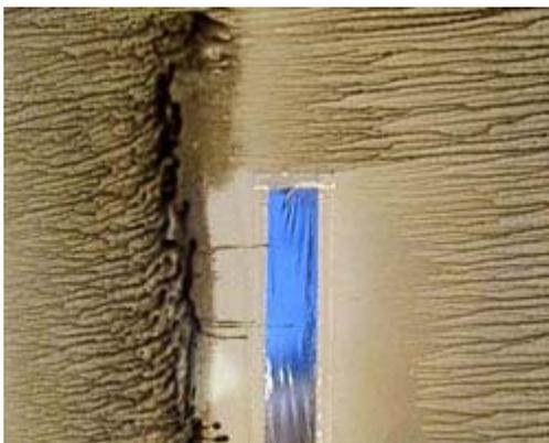
**Fig 1b. Photograph of FCSD strip on wing showing effect on near surface flow visualized with oil (Flow is from left to right)**
