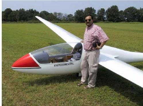
**Fig 5. The Standard Cirrus, 15-m wingspan, single seat, all composite test sailplane**
