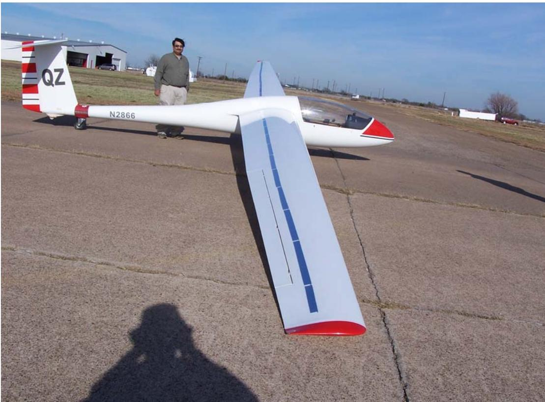
**Fig 9. Full-Span upper surface Deturbulator on Std. Cirrus as evaluated by Johnson<sup>19</sup>. (50-mm wide Deturbulator Tape with Vents between 200-300 mm long segments)**
