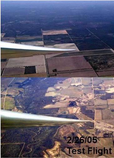
**Fig 8. Clean wing 30° bank (top) versus 60% inboard span FCSD treated 45° bank (bottom). Lower wing deflection even under higher loading (bottom) is due to increased lift from inboard sections.**
