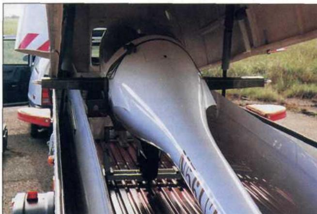
The SZD-56-1 loaded in its trailer. Note that the wing carry-thru spar, which is permanently attached to the fuselage, extends about 18 inches beyond the fuselage sides. Therefore, to keep the trailer from being overly wide, the fuselage is stowed somewhat elevated on its support dolly with the fuselage spar above the wing trailing edges.
