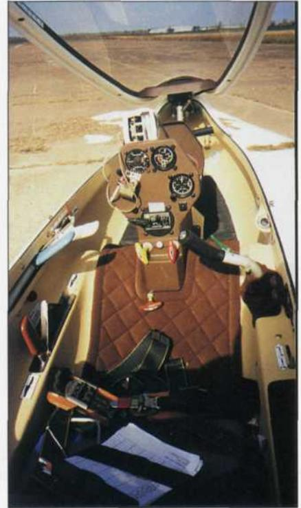
Cockpit view with control stick on upper right side, airbrake handle on upper left side aft, flap handle on upper left side forward, and landing gear handle on lower left side. Note the Rico Drag meter temporarily mounted at the top of the instrument panel, and the electric instrument vibrator temporarily mounted on the left side of the instrument panel.
