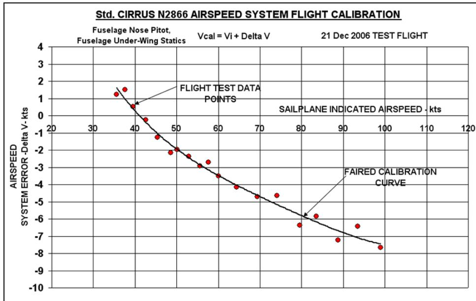
**Figure 3. Airspeed System Errors**
