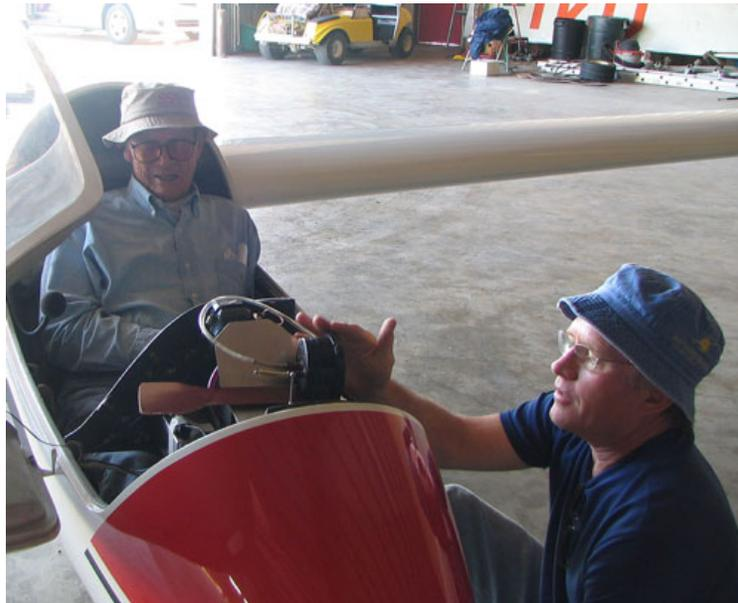
**Figure 10. Dick Johnson and Jeff Baird calibrating the airspeed indicator**
