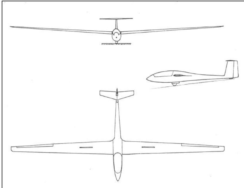
**Figure 1. Three-View Drawing of Standard Cirrus Sailplane**
