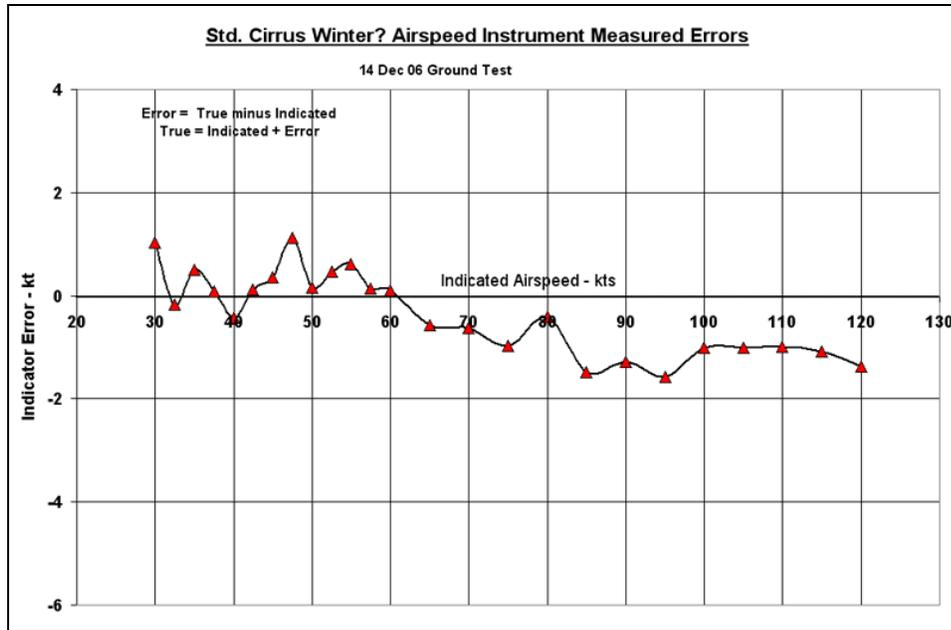
Figure 2. Airspeed Indicator Instrument Error
